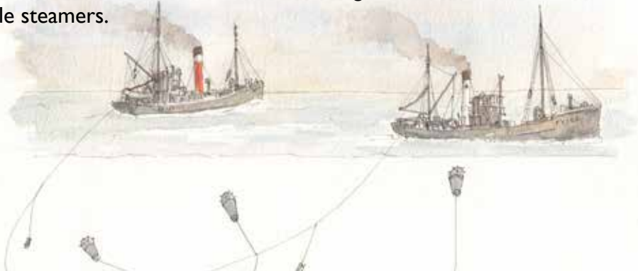
A pair of steam drifters work together to clear mines. A sweep-wire suspended between the boats (beneath the water) could snag and cut a mine's mooring rope. The mine would rise to the surface where it would be detonated by gunfire from the drifter. Painting by Mike Greaves
