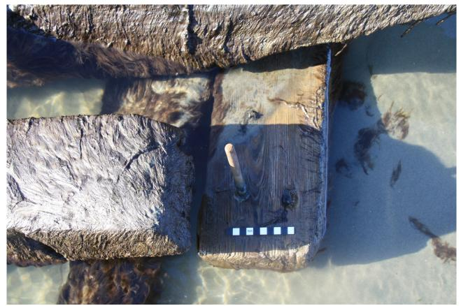
Figure 12. Planking butt end containing a retained copper fastening bolt. A hole for a second (upper) bolt is to the right (scale = 10cm).
