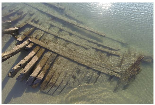
Figure 7. The stern of the vessel at northern end of the wreck, looking west. The stern post is visible at the righthand side of the picture. Third-futtocks and top-timbers have been trimmed off flush with one another. This area of structure would have originally been far more vertically aligned but has fallen outboard, to lie flat on the seabed.
